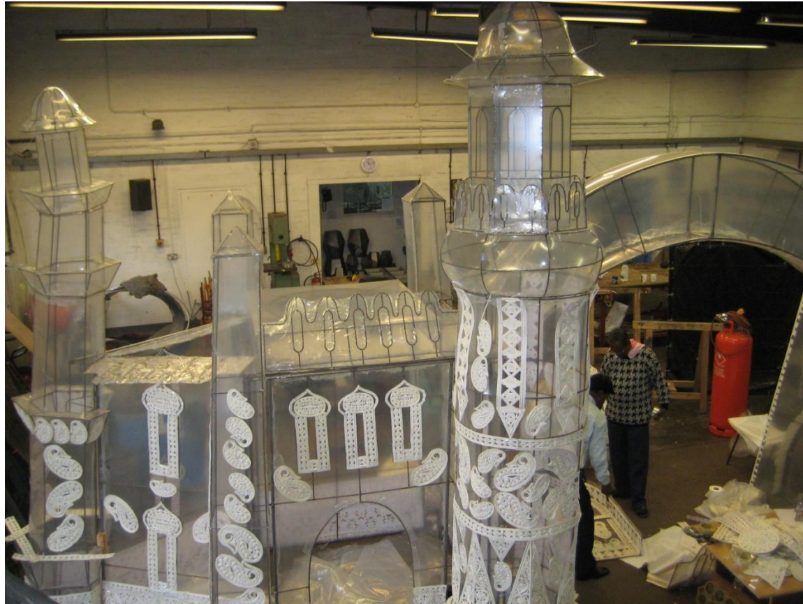
The Armature being Clad with Shola panels
